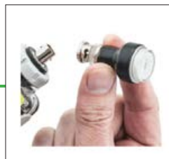
MAC004 strobelight attachment for verifying run speed
