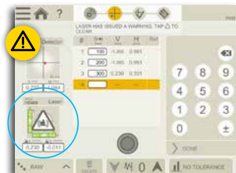
The built-in sensors warns on the display on events which can affect the measurement reliability.
