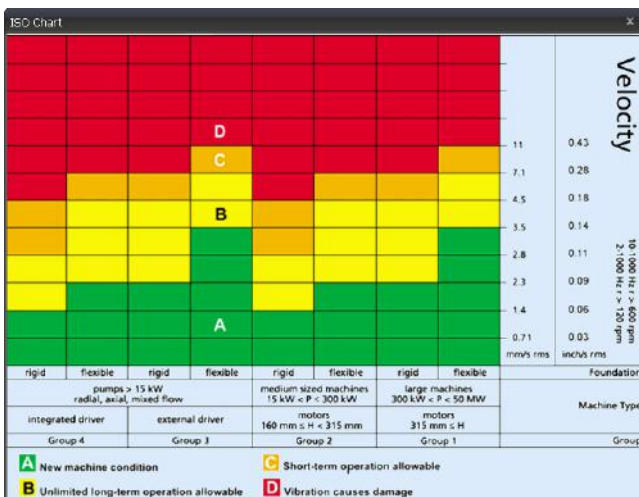
ISO 10816-1:1995. Mechanical vibration - Evaluation of machine vibration by measurements on non-rotating parts.
