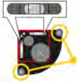
Level the laser transmitter
