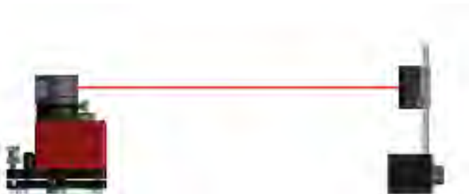
5-10 m between laser and detector
