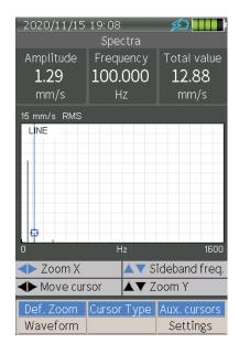
• Save Saves a measured spectrum file in the SD memory card. It can be opened later in file menu or transferred to PC software to be analyzed.
