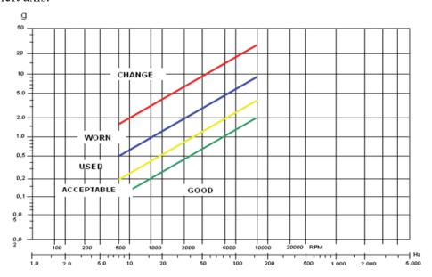
The figure above is a guide to interpreting the bearing condition value. If vibrations from other causes (e.g. flow surge and sometimes gear mesh forces) have vibrations within the frequency range, this can indicate a high bearing condition value without the bearing being damaged. A high bearing condition value can also be acquired if the bearing is poorly lubricated or is overloaded due to a large misalignment or a large belt tension.
