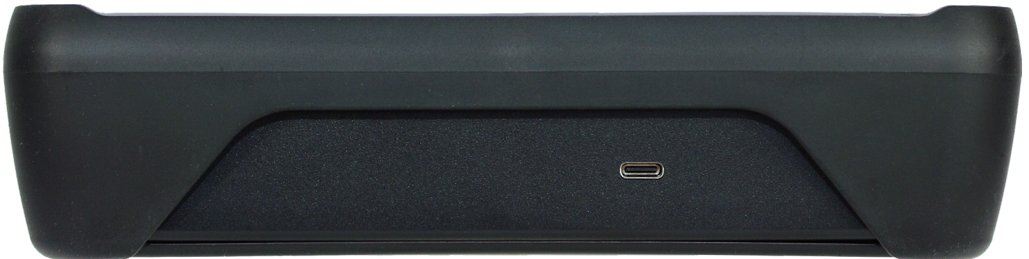
Back view containing USB Type - C for fast charging and communication with the application in the PC
