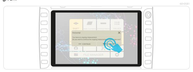
6. Enter the measurements **S-M**, **RPM**, **M-F1** and **F1-F2**. *Tips! Measure from the center of the rods for S-M and M-F1*.
