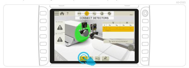
13. In this example we use *EASYTURN* method, place the detectors in a green area (*ONLY rotate the detectors by holding the shaft*) *Do not block the laser beam!* and press the green button, on the screen or on the XT12. Repeat the step for all green positions, at least three points are needed.
