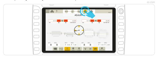
17. Write down, or take a screenshot of, the values for the shims *before* you loosen the bolts, *these values change when the bolts are loosened*..Loosen the bolts on the motor.
